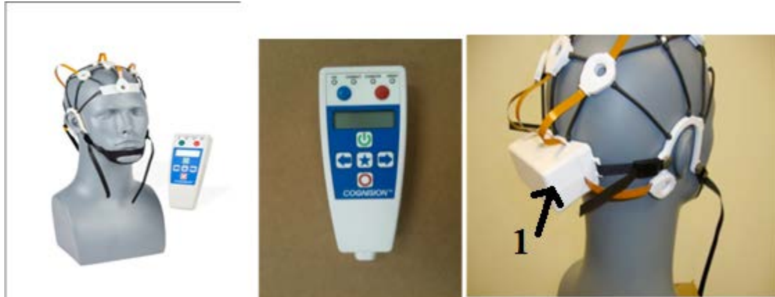
FIGURE 4 : The COGNISION™ 3000 Consists Of (A) Ten-Electrode Headset, (B) Control Unit, And (C) Data Acquisition. The Ubeyoke (1. White Box) Contains Electronics For Signal Amplification, Analog-To-Digital (A/D) Conversion, And Control Logic (C).
