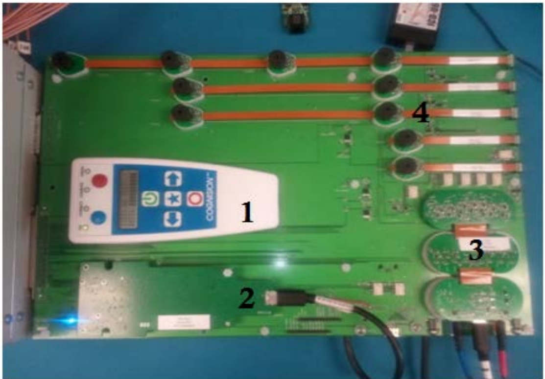
FIGUER 10 : Test Board With 1.HCU TOP, 2.HCU BOTTOM, 3.Uberyoke, And 4.Electrode Strings In Position. This Is A PCA Test Fixture That Allows The Unassembled Components Of The CS System To Be Mounted And Tested.
